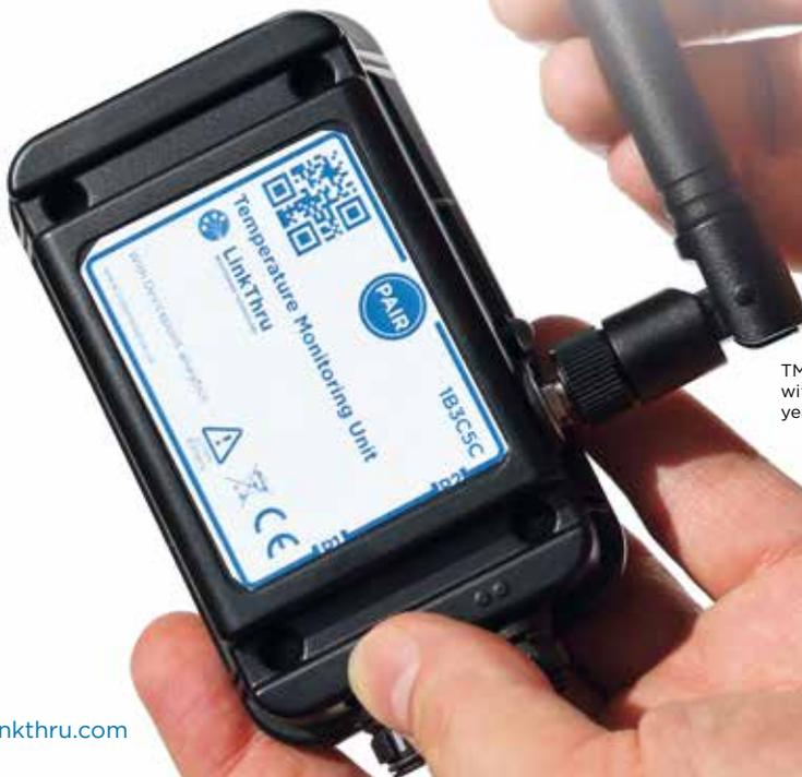
TMU devices are battery-powered with a long life of between 3 and 5 years, depending on the data mode.
